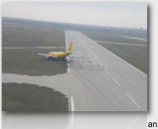
increasingly strong vibration. As it decelerated to 85kt, and the thrust reversers were stowed, the aircraft veered left.
